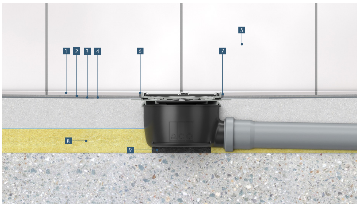
Installation proposal ACO sanitary gully Easyflow+ (floor construction according to sound insulation test report)
